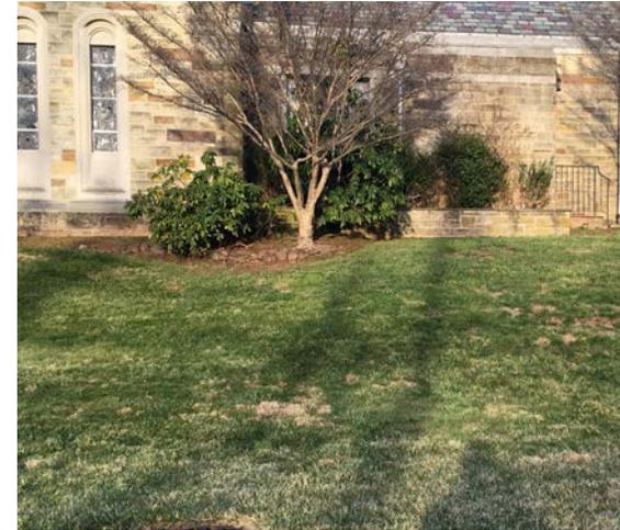
Two rain gardens can be installed in the front lawn of the building to capture stormwater from the rooftop of the building. Additionally, pervious pavement can be installed in the parking spaces to capture runoff flowing down the pitched driveway area. A preliminary soil assessment suggests that more soil testing would be required before determining the soil's suitability for green infrastructure.
